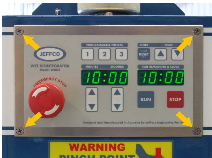
Remove the four screws holding the Control Panel on.
